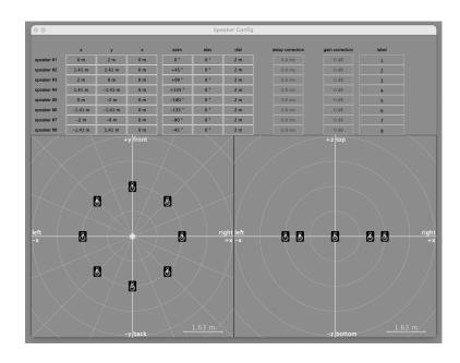
Move a speaker in the lower panel to quickly adjust its position.
