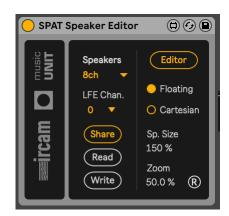
LFE" stereo pair. LFE channel in 5.1 or 7.1 setups is often set to channel 4. Setting the value to 0 removes the dummy channel. Note that SPAT devices don't provide integrated bass management.
