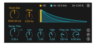
initial level, after an interruption of the input signal. The decay time is controlled in the same way as an equalizer curve, either globally or in three separate frequency bands with controllable transition frequencies, and can be varied from 0.5s to 30s.
