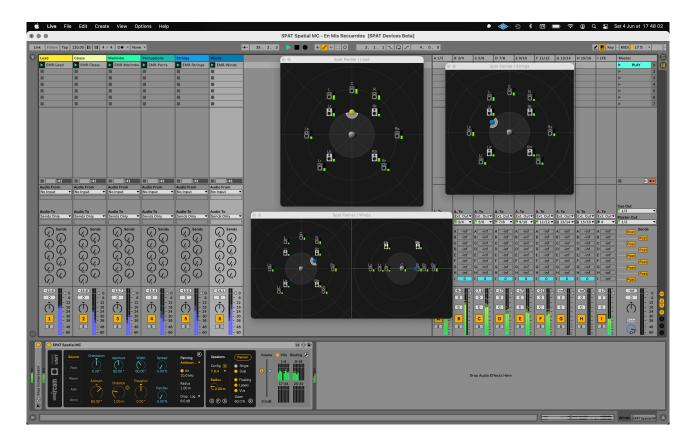
The device can feed sound systems with up to 32 satellite speakers, and allows to select a speakers configuration among a collection of presets corresponding to most popular speakers setups, from simple quadriphonia to standard 5.1 or 7.1, up to more complex Dolby Atmos-compatible setups. The sound source's position and radiation can be graphically manipulated in a floating panner window, which interacts with navigational coordinate parameters such as azimuth, distance and elevation.
